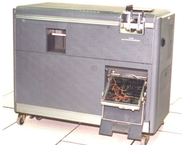
The IBM 602 Calculating Punch (1946)
